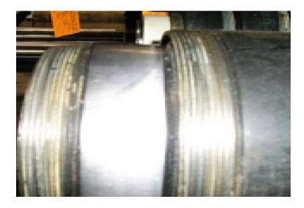
A cylinder that has taken a bulge, similar to the one in this picture, is an issue that needs to be taken care of immediately. The driver of the truck in this picture was lucky as the only cost was the replacement of the cylinder.
