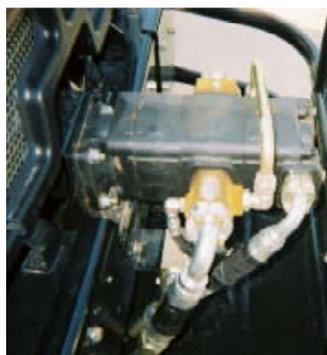
Parker's HOC system shown above with tandem bushing pump to power automated side loaders.
